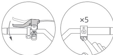
EN Turn the scooter on. Make sure the scooter is not locked or during charging, squeeze the brake lever and simultaneously press the accelerator 5 times, when the display is off, the scooter has been restored to factory settings, and the scooter cannot be searched for by the Find My app. If you need to pair again, delete the added scooter from the Find My app and then pair it again.
