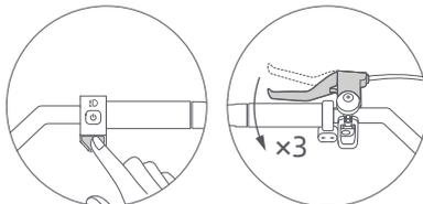
EN Press the accelerator and squeeze the brake lever 3 times to activate the scooter's serial number search function. The serial number will then be displayed in the Find My app (for iOS users who have paired the scooter using the Find My app).
