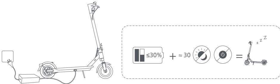
EN The scooter is fully charged when the LED on the battery charger changes from red to green.
