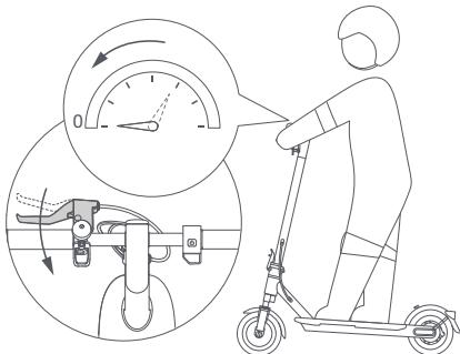
**EN** Release the accelerator to slow down, and press the brake lever to brake.
