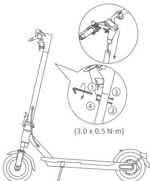
EN Put down the kickstand, and hold up the stem until it is completely in an upright position. Then push the quick release lever inward to the end.
